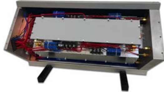
Figure 1: The CRE-350D-1 RF Module (cover removed).
