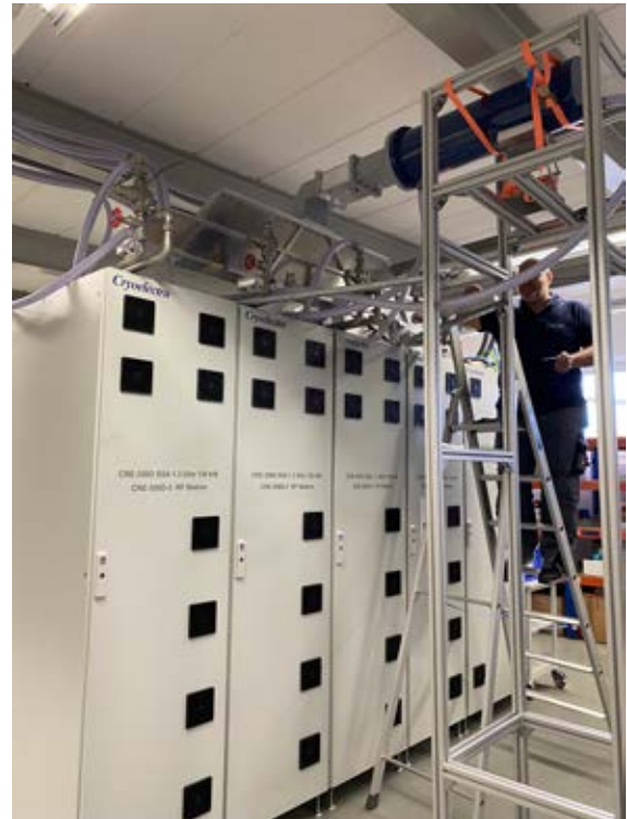
Figure 5: CRE-350D Solid-State Amplifier during Factory Acceptance Test on a Water Load
